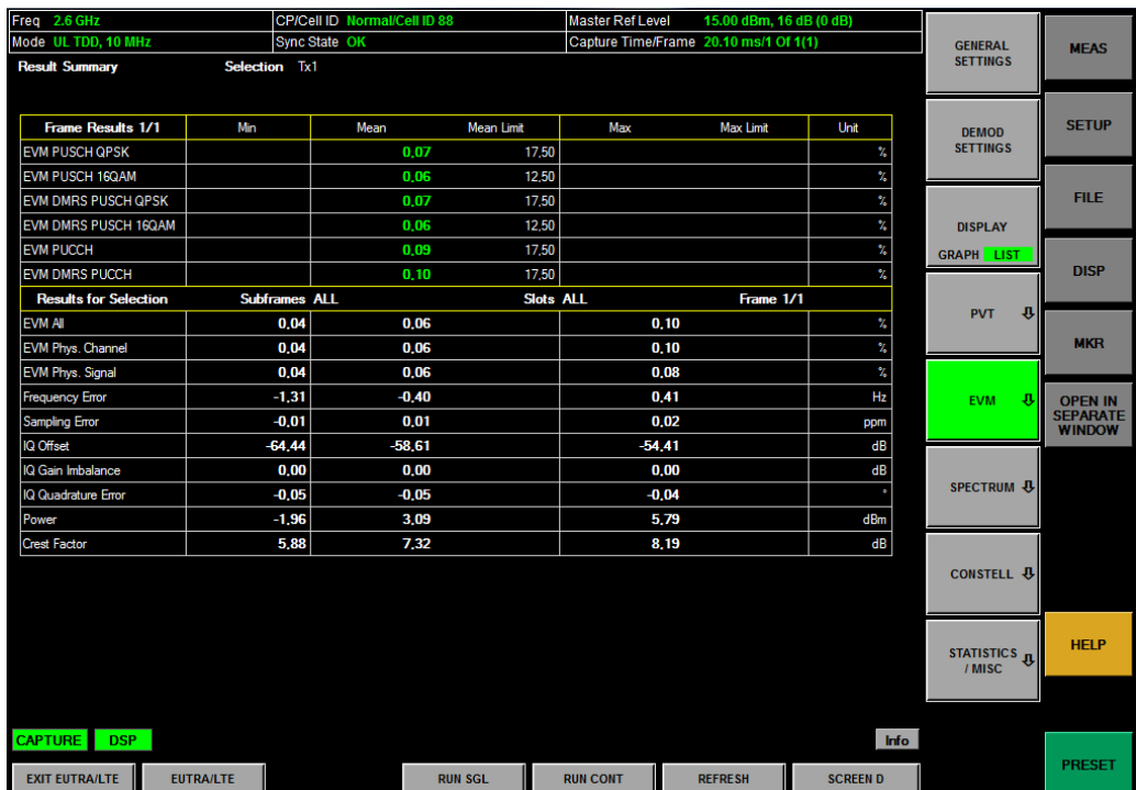
Figure 2-36: EVM measurements in tabular format for one selected TX antenna in single screen view
