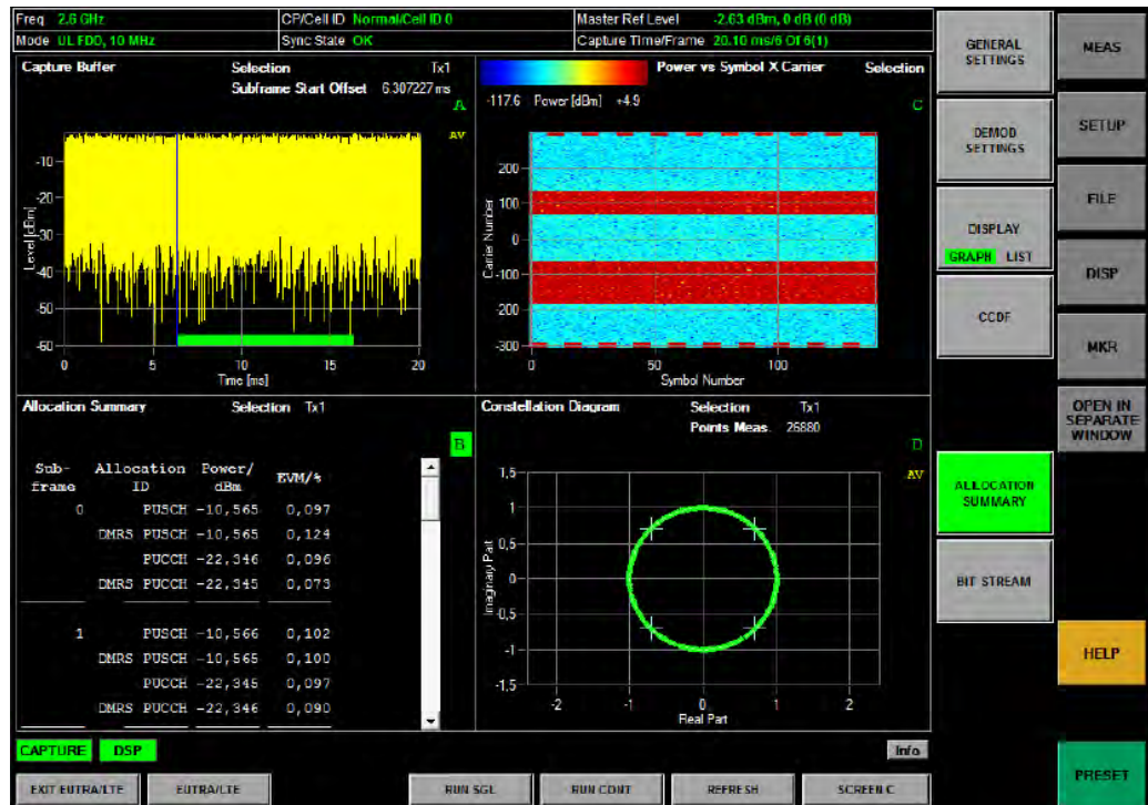
Figure 2-29: Enhanced SC-FDMA measurement using FS-K10xPC software for FSW
