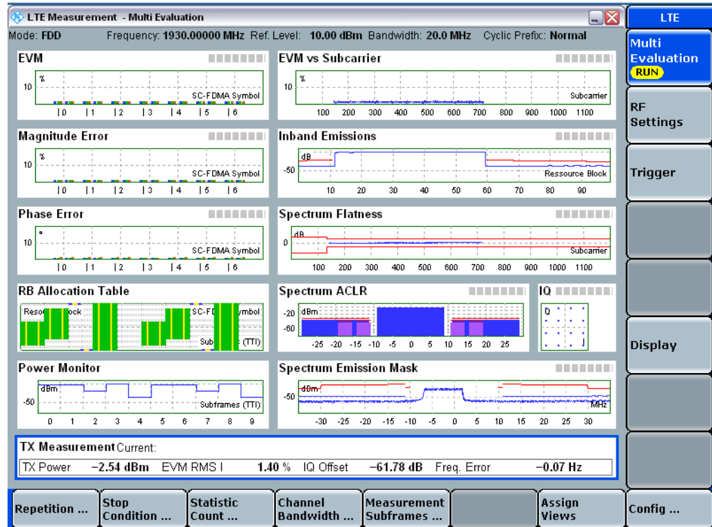
Figure 2-42: Tx measurements of a DUT uplink signal using CMW500
