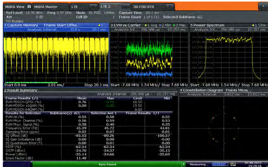
Figure 2-23: LTE measurements on a single component carrier using FSW-K100
