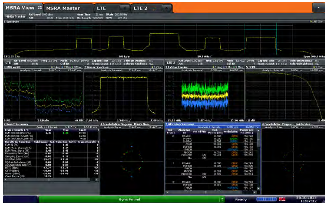
Figure 2-27: MSRA view with different measurements on two of the five components
