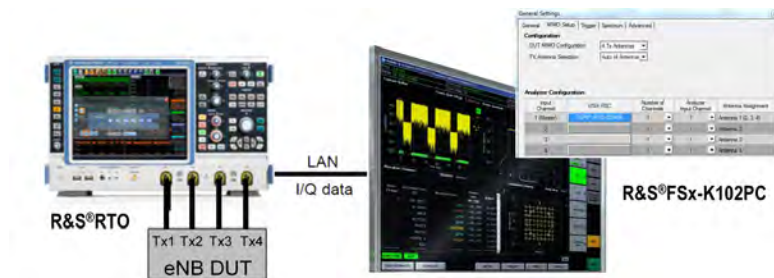
Figure 2-31: Test setup with an RTO for measuring a MIMO signal
